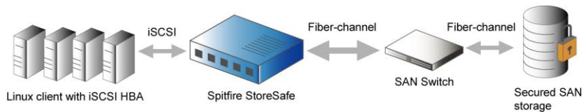
Figure – FC-SAN test with Bloombase Spitfire StoreSafe Security Server for SAN protection
