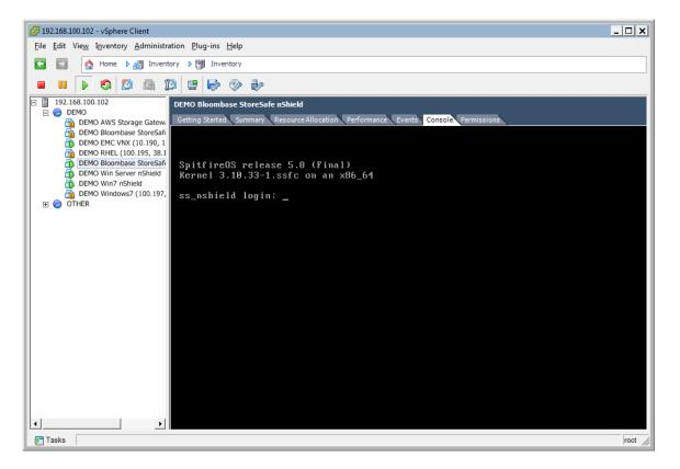
Bloombase StoreSafe software appliance is deployed as a virtual appliance (VA) on VMware ESXi.
